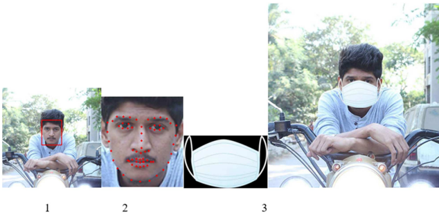
Fig. 6. Creation of the synthetic dataset. Step 1 – face detection; Step 2 - facial landmarks detection. Step 3 – Drawing on top of the original image a surgical mask. As taken from [10].
