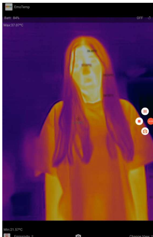
Fig. 1. Example of automatic finding of the points with the highest temperature. Warning when a value is above the set threshold temperature (here it was set at 37.0 degrees Celsius). The temperature point from the nose turned red.
