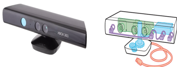
Fig. 9. Internal components of Microsoft Xbox 360 Kinect
