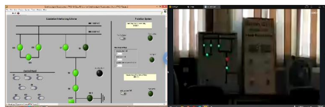
Fig.8 Interlocking Schemes Practical Experiment Using LabVIEW and View from the Lab.
