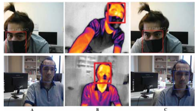
Fig. 1. The detected object from two different input images from the RGB camera and thermal camera. A) The output of Module 1 detects the position of the mask and classifies it into the corresponding class label with a confidence score. B) Detected “head” label of output image in Module 2 from the thermal camera. C) Output image of Module 3. A combination of the mask-wearing position and head temperature of the detected head are combined into a single output image containing object prediction and object temperature
