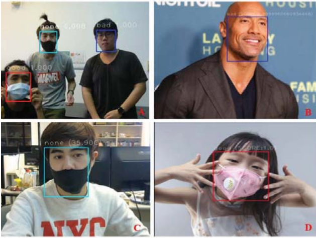
Fig 3. Sample of detected images from different angles and different y class labels of mask-wearing positions. A, C) Images captured from real-time RGB camera with all classes of mask positions. B, D) Classification images from the testing dataset with class label predictions.
