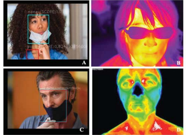
Fig 4. Sample of the failed detected images from Module 1 and Module 2. In A, C) our model gives two high confidence scores for different classes. In B, D) Module 2 fails to detect the different quality images from another output camera.
