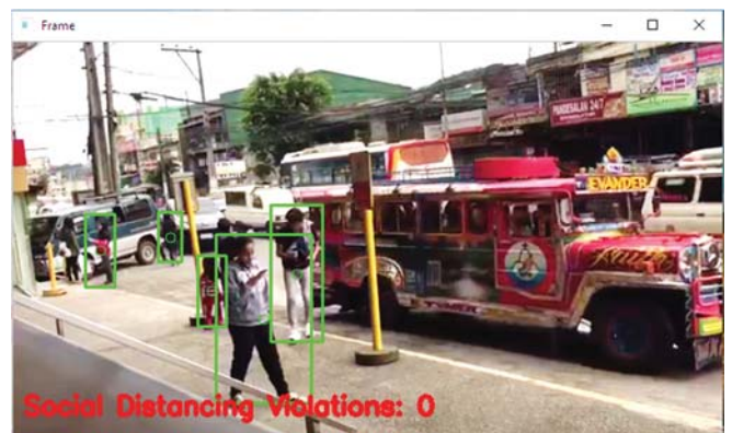
Fig. 11. The output result of a picture with persons observing the social distancing mark with the green color.
