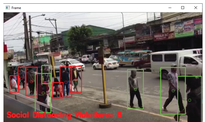
Fig. 10. The output result of a picture with six persons violating the social distancing mark in the color red.
