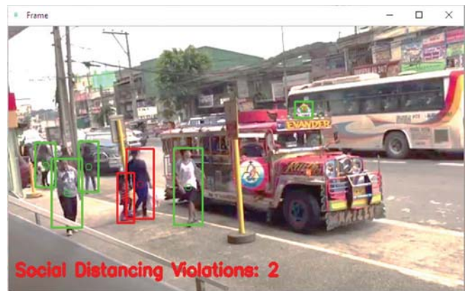
Fig. 9. The output result of a picture with two persons violating the social distancing mark in the color red.
