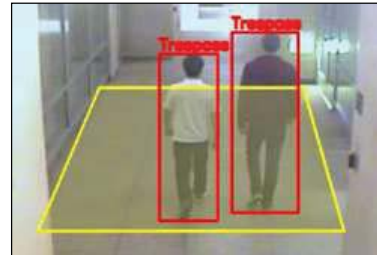
Fig. 11. Red bounding boxes with the word “Trespass” indicate an alert or warning when entering the ROI.
