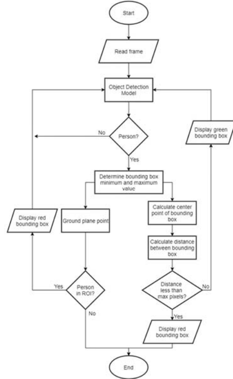
Fig. 3. Person detection for social distancing and safety violation alert based on segmented ROI flowchart.
