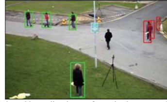
Fig. 9. Multiple red bounding boxes for a single person show the object detection fails to locate person accurately on dataset PETS2009.
