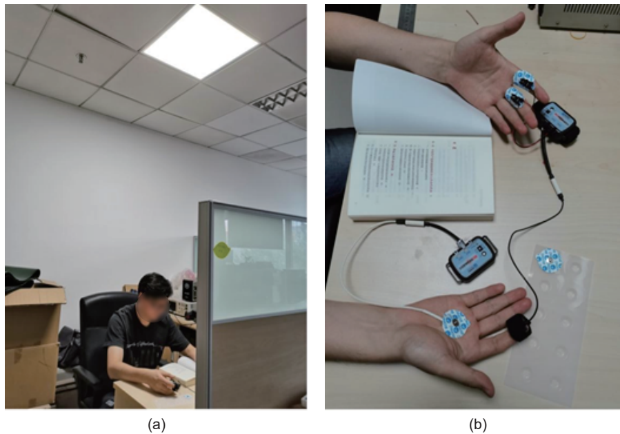
Fig. 11 Light stroboscopic irradiation experiment with (a) the setup of the environment having irradiation light from the ceiling and (b) the measurement on hand while the volunteer is reading.
