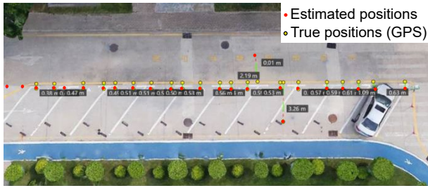
Fig. 4 Tracking of a walking pedestrian, where the GPS coordinates are depicted in yellow dots, estimated positions are represented by red dots, and errors are marked in tags.
