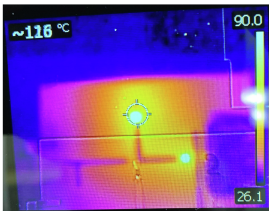
FIGURE 23. Temperature profile of the two diodes of the fabricated charge pump rectifier.
