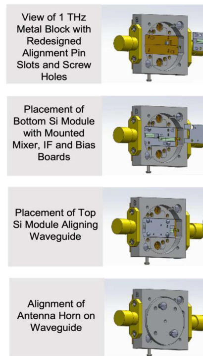
FIGURE 2. Visualization of assembly process utilizing a model of the 1 THz block secured with metal interface, where several of the main parts of the extended process is shown from top to bottom.
