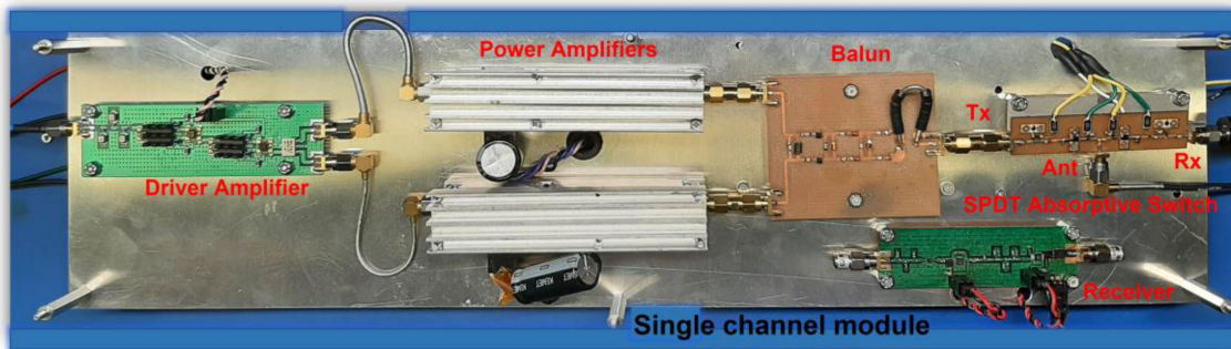
FIGURE 14. Single channel module of the UWB Radar.
