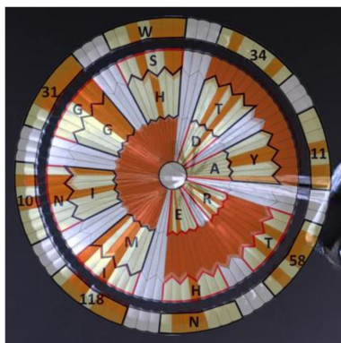
FIGURE 1. View of parachute underside on the Perseverance rover with overlaid coded message text. Each of the three inner rings of white and red lines represents a 7-bit binary code spelling out “Dare Mighty Things” going clockwise with A = 000001, and with the outer ring spelling out the Lat. and Long. of JPL’s Visitor Center. Image NASA/JPL, 2021: https://mars.nasa.gov/imgs/mars2020/spacecraft/markings/25646_PIA24431-parachute-decoder-ring-1200.jpg .
