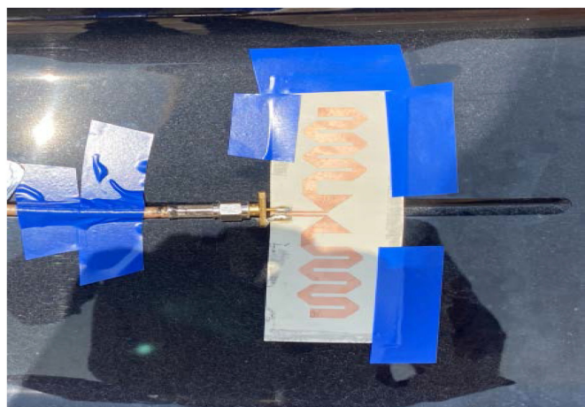
FIGURE 20. Antenna placed on the trunk lid of the vehicle.
