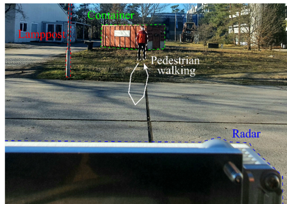
FIGURE 33. Measurement scenery with a moving pedestrian. The radar faces several obstacles such as a lamppost and a container. The path of the pedestrian is outlined by a white arrow.
