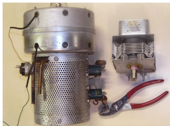
FIGURE 7. Photo of older Raytheon water cooled QK707 magnetron and redesigned and miniaturized version of the QKH1381 air cooled magnetron tube for 2450 MHz. From [46] page 47. ©IEEE, with permission.
