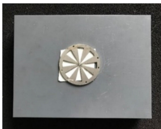
FIGURE 5. Test object: Siemens star on PVC plate. Plate dimensions: 20 cm x 15 cm, depth 3 cm. Star dimensions: diameter 6 cm, thickness 1.5 mm. The object is scanned so that the Siemens star is on the plate's backside, not facing the antenna array (i.e., photograph displays rear view of scanning scene). The Siemens star was stuck to the PVC plate with adhesive tape (white rectangular area in the picture). Due to the small thickness of the adhesive tape, it has no noticeable effect on the imaging result.
