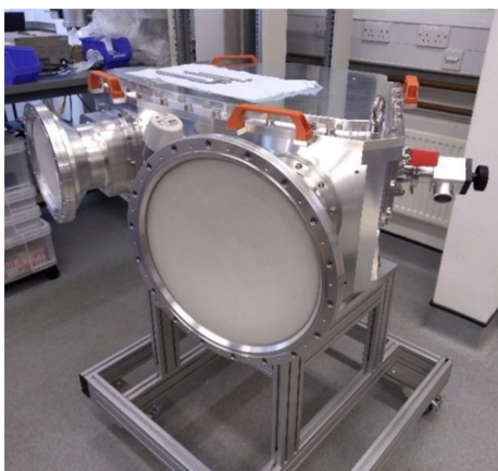
FIGURE 20. Band 345(6) prototype cryostat ready for assembly and integration at the University of Oxford.
