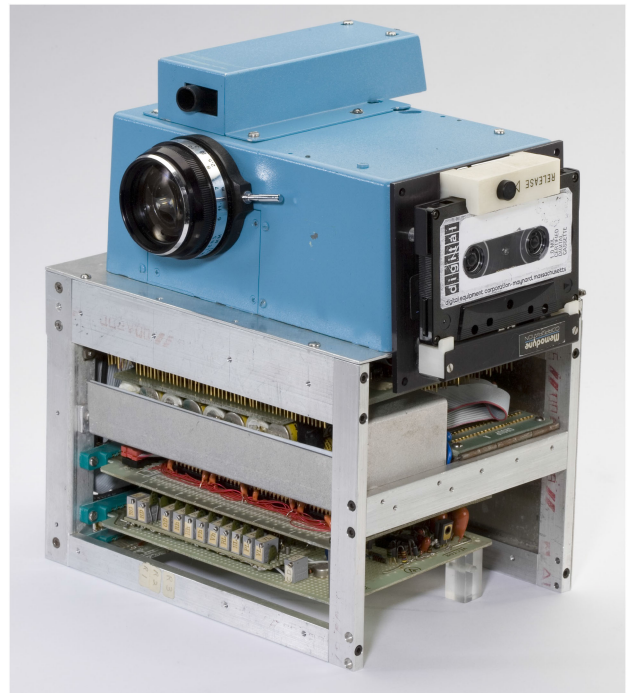
FIGURE 1. First compact digital camera invented in 1970s. The picture size was 100x100 pixels and the data was recorded on a cassette tape. (Courtesy of the George Eastman Museum with permission from Eastman Kodak Company).
