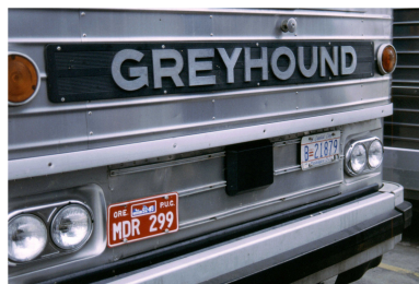
FIGURE 2. 24 GHz VORAD radar mounted at the front side of a Greyhound bus. Photograph by W. Menzel.
