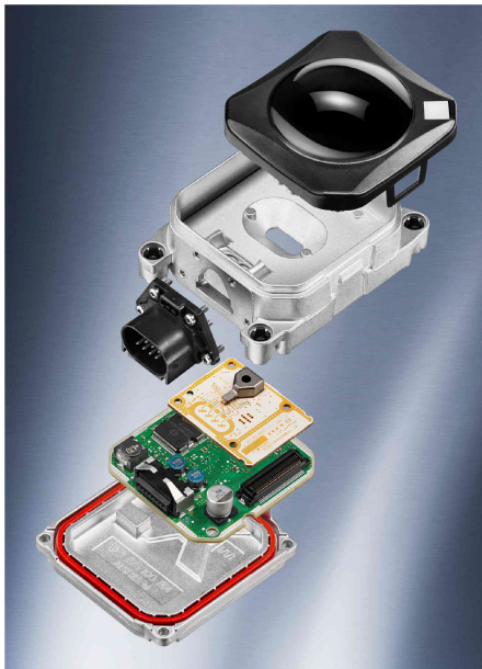
FIGURE 5. Exploded view on the Bosch LRR3 sensor and details of the planar antenna elements feeding the lens. Sensor photograph provided by Bosch.
