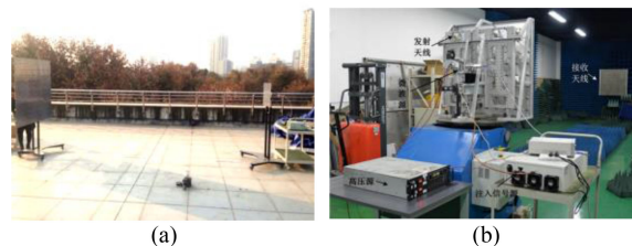
FIGURE 26. Chengdu microwave power beaming experiments at (a) 2.45 and (b) 5.8 GHz.
