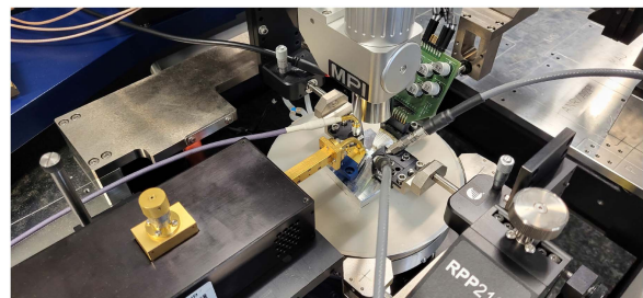
FIGURE 16. Photograph of the measurement setup for receiver testing. Left: VNA-X with WR 6.5 GSG probe; Bottom: GSSG RX mixer output; Top: VCO mixer divider output; Right: DC supply.
