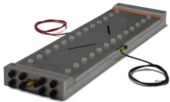
FIGURE 18. Manufactured test fixture with slotted cover plate [77].
