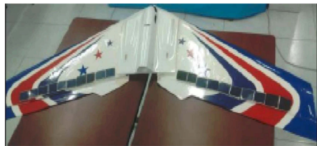
FIGURE 23. Prototype of UAV with monocrystalline solar cells mounted in the wings as presented in [140].
