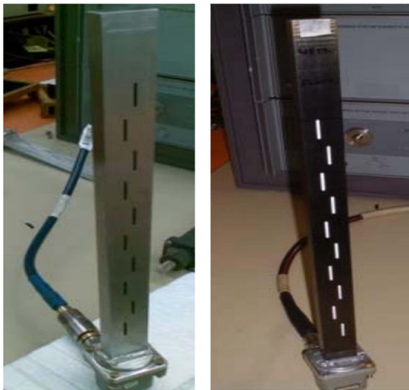
FIGURE 19. Photographs of the aluminum (left) and CFRP (right) 10-slot slotted waveguide antennas (SWASS) [70].
