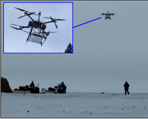
FIGURE 19. Ku-band radar mounted on a drone and operating long-range flights in Utqiagvik, Alaska.
