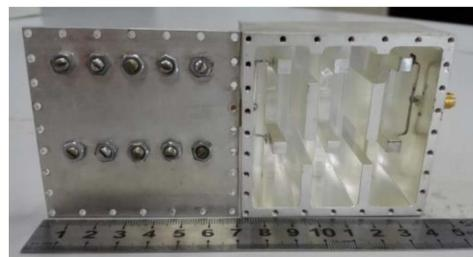
**FIGURE 8.** Photograph of the fabricated dual-band bandpass filter.
