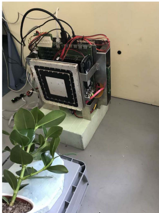
FIGURE 14. Measurement setup consisting of millimeter wave MIMO imaging radar and the plant onto which the insect was placed.
