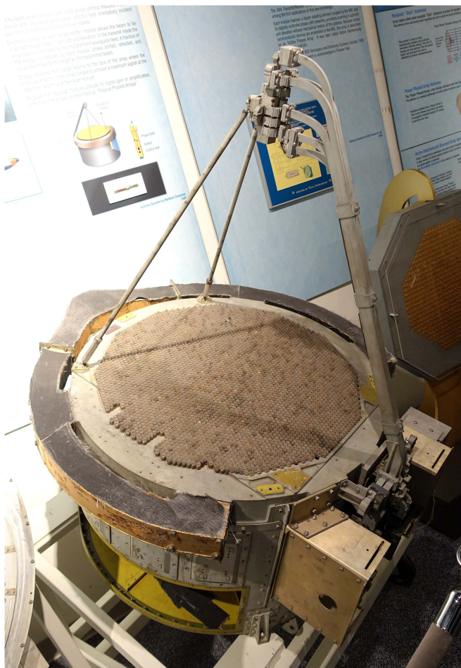
FIGURE 6. RARRF, antenna reflecting array radio frequency, raytheon, 1968-1969, Ku-band, with over 3500 phase shifting modules.
