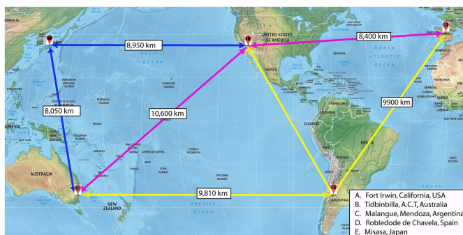
FIGURE 1. Present global X/Ka VLBI network. JAXA's Misasa, Japan 54-meter, and ESA's Malargüe, Argentina 34-meter station are recent additions to the X/Ka network adding valuable new baselines with added sensitivity.
