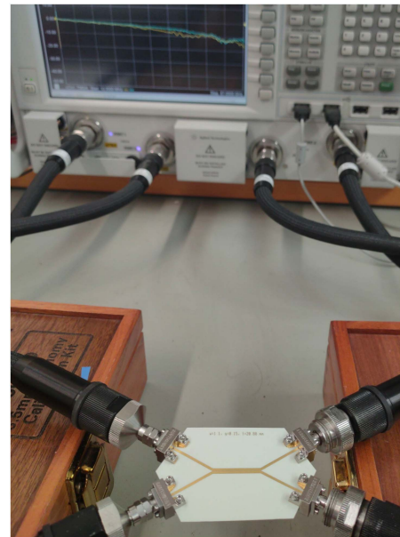
FIGURE 9. Photograph of manufactured coupled lines and the measurement setup using vector network analyzer for Pure Mode S-parameters measurement.
