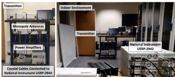
FIGURE 10. Photo for the closed-loop WPT system prototype and experiment in the indoor environment.
