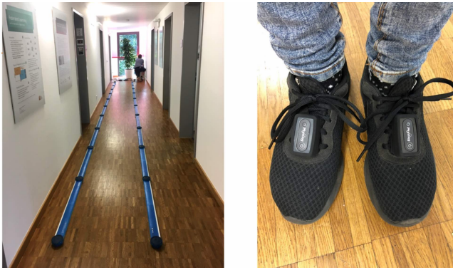
Fig. 1: Experimental Setup. Left: the 10-meter OptoGait walkway. Right: the IMUs were fixed on top of the shoes.
