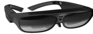
Fig. 1: ODG R7 smart glasses. The smart glasses had a Qualcomm Snapdragon 805 2.7 GHz quad-core processor, a monocular camera, diagonal 30-degree field of view, 10-degree vertical field of view, a Bluetooth link, and an Inertial Measurement Unit (IMU) sensor.
