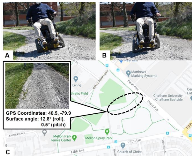
Figure 5. MEBot navigating over uneven terrains using passive suspension similar to EPWs (A) compared to MEBot using its self-levelling seat application for tip prevention (B). The MEBot's sensor package sends the location and surface angle to the eNav-Server (C).
