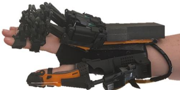
Figure 1: HandMATE device. Individually actuated fingers and thumb shown. Electronics box is affixed to back of splint.
