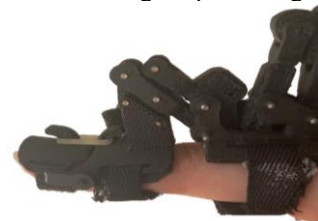
Figure 3: Additional proximal finger segment with passive elastic assistance.
