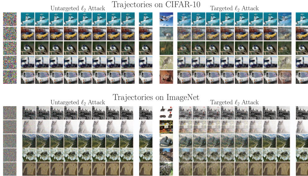
Figure 7: Visualized trajectories of HopSkipJumpAttack for optimizing \ell_2 distance on randomly selected images in CIFAR-10 and ImageNet. 1st column: initialization (after blended with original images). 2nd-9th columns: images at 100, 200, 500, 1K, 2K, 5K, 10K, 25K model queries. 10th column: original images.
