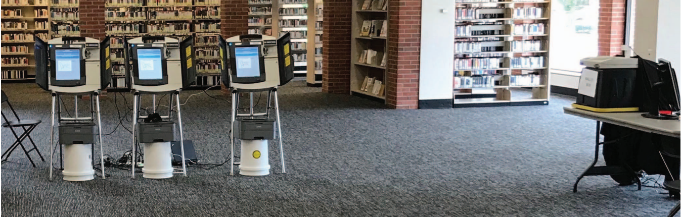
Fig. 1: Polling Place Setup . We established mock polling places at two public libraries in Ann Arbor, Michigan, with three BMDs ( left ) and an optical scanner and ballot box ( right ). Library visitors were invited to participate in a study about a new kind of election technology. The BMDs were DRE voting machines that we modified to function as malicious ballot marking devices.
