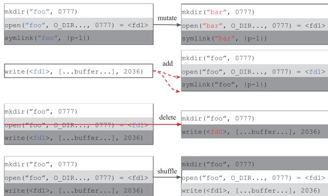
Fig. 4: Illustration of four basic syscall sequence evolution strategies supported in KRACE: mutation, addition, deletion, and shuffling. For KRACE, each seed contains multi-threaded syscall sequences and each thread trace is highlighted in different shades of grayscale.
