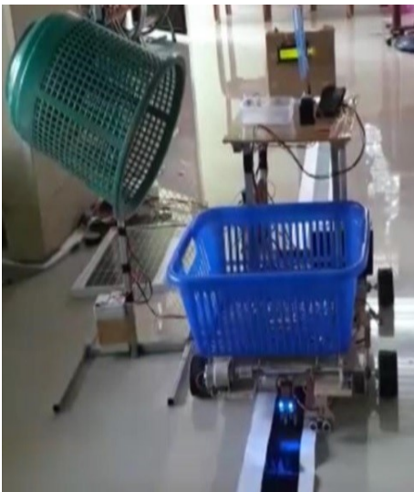
Fig 7: Waste collection mechanism of AGV system
