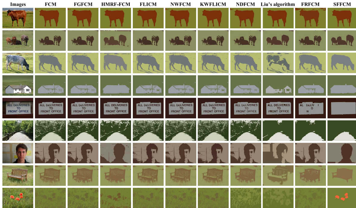
Fig. 14. Comparison of segmentation results on color images from MSRC using different models ( c = 2 ).
