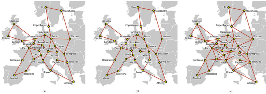
Fig. 2. EU network topologies used for the case studies, which all comprise 28 nodes: (a) basic topology, with 41 bidirectional links (the base topology from [50]), (b) sparse topology with only 34 bidirectional links (the ring topology from [50]), and (c) dense topology with 60 bidirectional links (the triangular topology from [50]).
