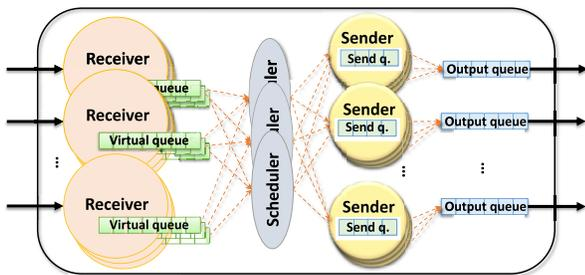
Fig. 6. Loop management architecture in LGCC routers.
