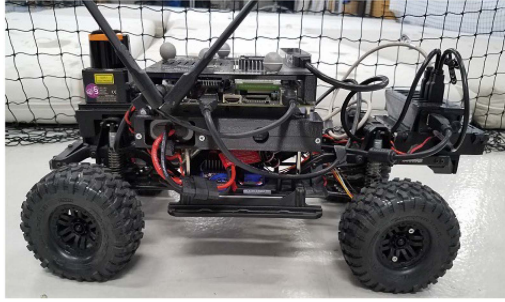
Fig. 4. SVEA vehicle based on an NVIDIA Jetson TX2 embedded computer used to evaluate the proposed solutions.
