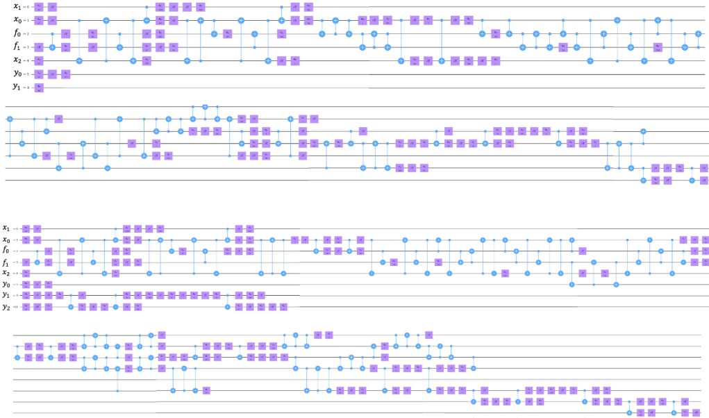
FIGURE 14. Our transpiled circuits of instance II (top) and III (bottom) to solve the DLP instance 2^z \equiv 2 \pmod{3} . The last observing gates are omitted.
