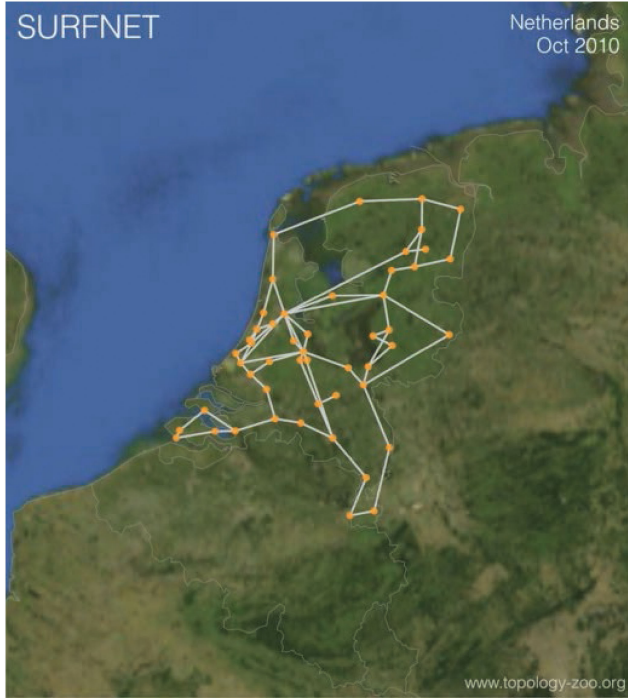
FIGURE 4. This figure is the graphical representation of the SURFnet network of Fig. 5. We run our rate maximization algorithm on this graph. Here, we consider the demand set as D = \{(40, 45, 7), (21, 13, 6), (30, 50, 7), (38, 15, 8)\} . The end-nodes are represented using hexagonal boxes. The capacity of each of the link is chosen uniformly at random between [1,400] -EPR-pairs per second. We assume that the success probability of the bell-state measurement is q = 0.5 and the fidelity of the each of the elementary pairs is F = 0.9925 and the value of the corresponding Werner parameter W = 0.99 . Given such a network and demand set, we run our edge-based formulation proposed in Table 1 and get a total achievable rate of 18.140625 EPR-pairs per second. Next, we feed the solution to the path extraction algorithm, proposed in algorithm 1 and extract the paths for each of the demands. In this figure, all the thick edges, participate in the paths. For the demand, (45, 40, 7) we get two paths, ((45, 43), (43, 47), (47, 48), (48, 9), (9, 33), (33, 40)) and ((45, 44), (44, 47), (47, 48), (48, 9), (9, 39), (39, 40)) . Note that each of the paths has path-length 6. Hence the end-to-end fidelity for this demand is \frac{1+3(0.99)^6}{4} = 0.955 . Similarly, for the demand (21, 13, 6) the extracted path is ((21, 27), (27, 28), (28, 25), (25, 20), (20, 31), (31, 13)) and end-to-end fidelity is \frac{1+3(0.99)^6}{4} = 0.955 . For the demand (30, 50, 7) , there is no path of length smaller than 8. Hence, this demand cannot be satisfied in this model. For the demand (38, 15, 8) , we extract four paths, ((38, 23), (23, 31), (31, 14), (14, 15)) , and ((38, 39), (39, 31), (31, 14), (14, 15)) , and ((38, 39), (39, 9), (9, 48), (48, 46), (46, 15)) , ((38, 39), (39, 9), (9, 6), (6, 48), (48, 47), (47, 43), (43, 15)) and the end-to-end fidelity for the paths are 0.97, 0.97, 0.9625 and 0.9475. If we use the prepare and swap protocol for generating EPR-pairs, along each of the paths, then we can achieve the total entanglement distribution rate of 18.140625 EPR-pairs per second.
