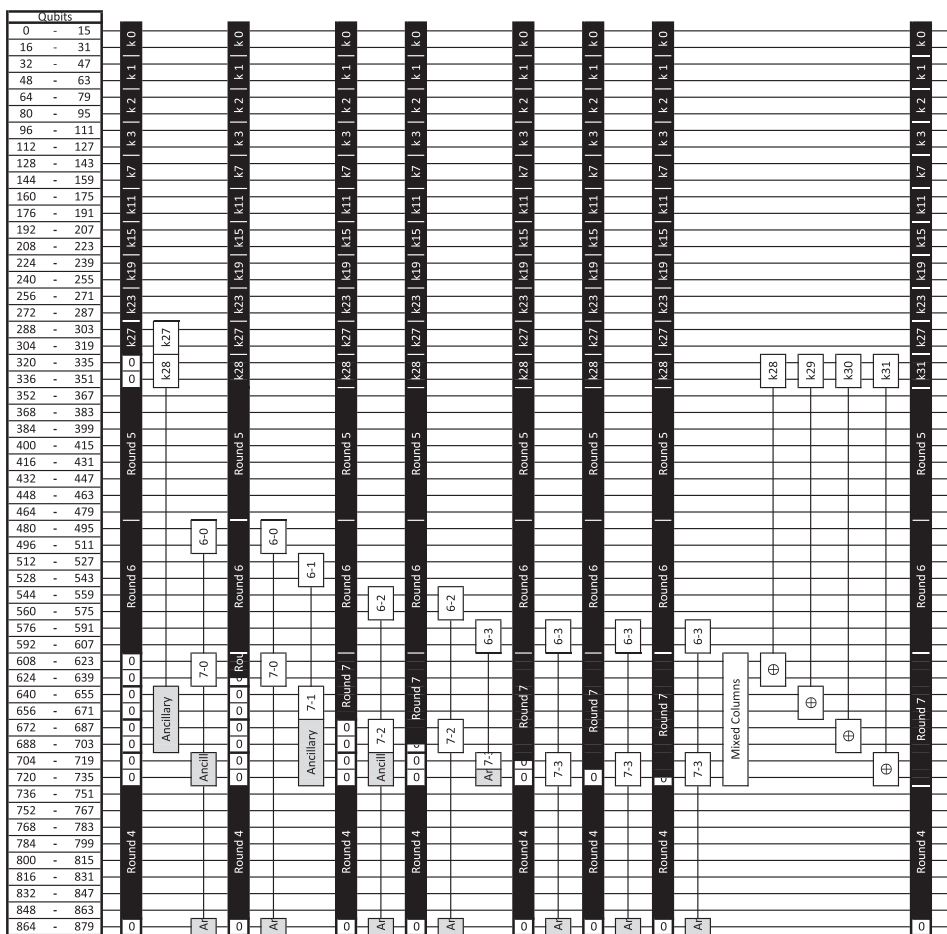
FIGURE 4. AES-128 diagram of Round 7 computations that have an S-box depth of seven. Each column represents an S-box depth of one.
