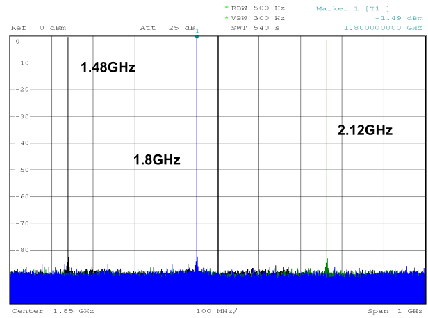
Fig. 10. Measured spectra of ADPLL output across the frequency operating range.
