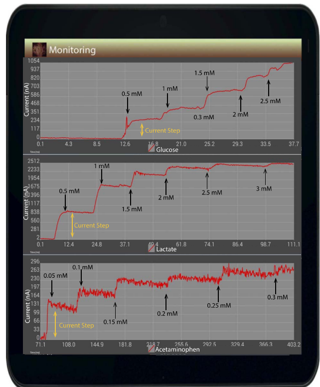
Fig. 1. Portable terminal showing real-time measurements for endogenous glucose and lactate and exogenous acetaminophen. Reprinted from [66].
