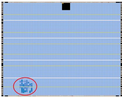
Fig. 11. Layout of the proposed architecture mapped on the Intel Cyclone IV E EP4CE115F29C7 FPGA (4 channels, L = C = 8 bits, A = 7 bits).
