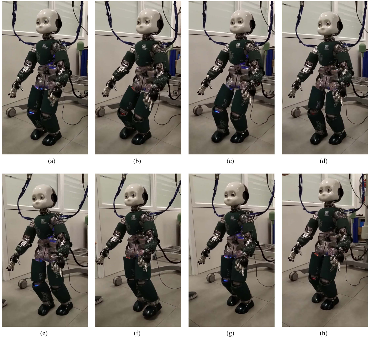
Fig. 5. Snapshots of the robot walking using the planned trajectories. The planner generates references which are interpolated and stabilized through a joint position controller. (a) t = t_0 . (b) t = t_0 + 1 s. (c) t = t_0 + 2 s. (d) t = t_0 + 3 s. (e) t = t_0 + 4 s. (f) t = t_0 + 5 s. (g) t = t_0 + 6 s. (h) t = t_0 + 7 s.
