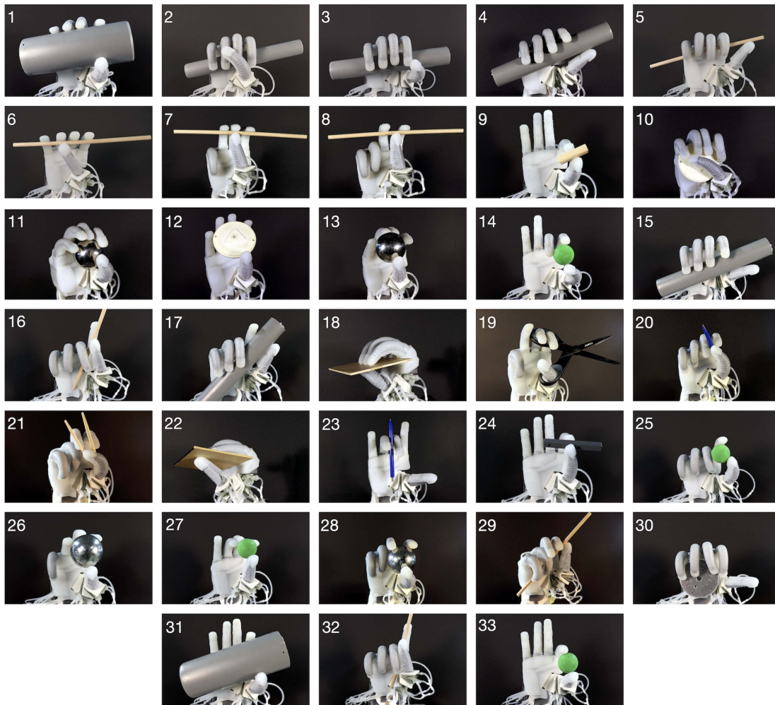
Fig. 10. RBO Hand 3 is able to replicate all 33 grasp postures of the most comprehensive GRASP taxonomy.
