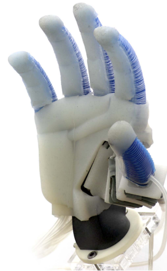
Fig. 1. Anthropomorphic soft robotic RBO Hand 3 with 16 independent degrees of actuation and a dexterous, opposable thumb based on pneumatic actuation. The soft actuators are slightly inflated to realize a natural looking posture of a relaxed hand.
