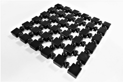
Fig. 4. 3-D printed prototype of a 6 \times 6 morphing cover skeleton with passive spherical joints designed with the proposed approach.
